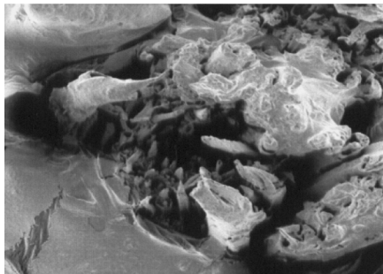
FIGURE 10 SEM micrograph showing date palm fiber embedded in high viscosity polyester composite.
